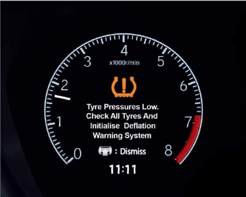
TYRE PRESSURE MONITORING SYSTEM (DEFLATION WARNING SYSTEM)
