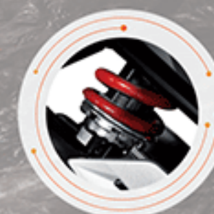
7-STEP ADJUSTABLE- REAR MONO SHOCK SUSPENSION
