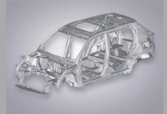
Advanced Compatibility Engineering (ACE™) Body Structure
